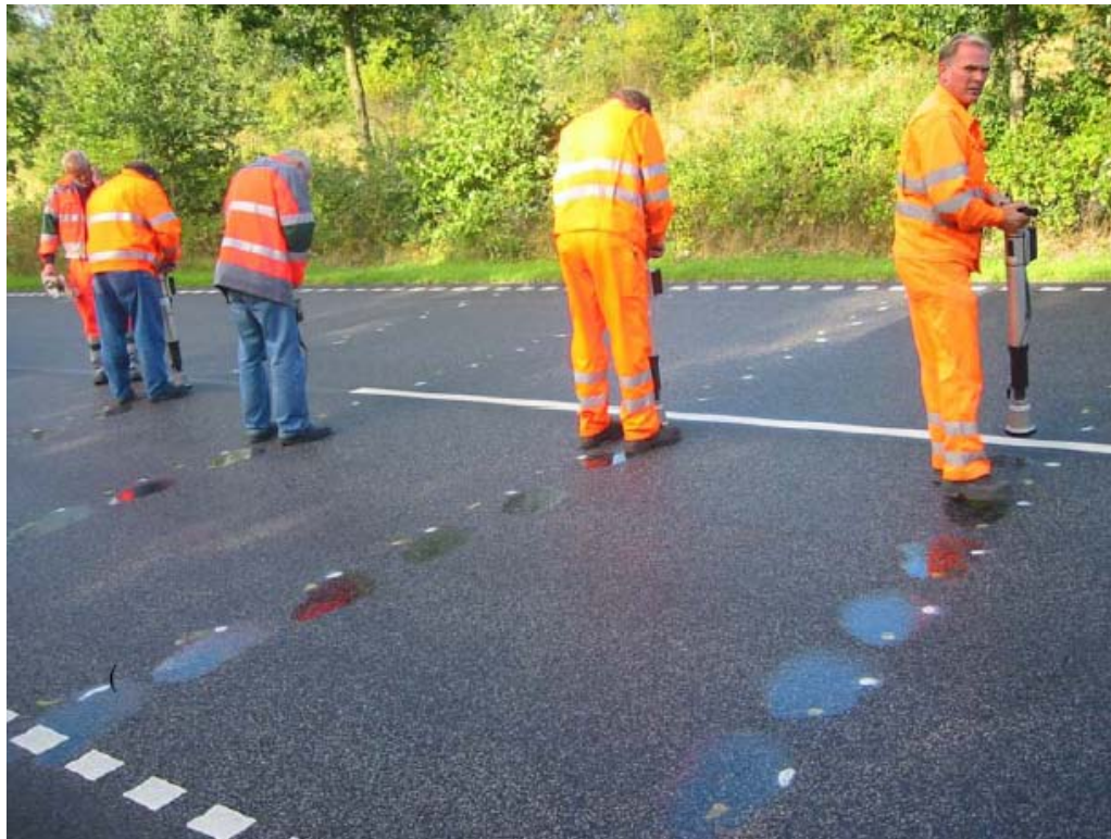
13 14 FIGURE 1 Measurements with SOBO20 portable salinity testers, 15 at each subsection five cross-sections 2 meters apart were measured by every 0.5 meter.
