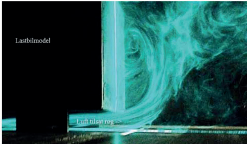
Example of vertical turbulence behind a truck. "Trafik og Veje", 2013, October, page 43
