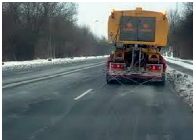
Nozzle spreader. The nozzles incline backward. Precision salt spreading. Private photo from Fyns Amt, January 25. 2006
